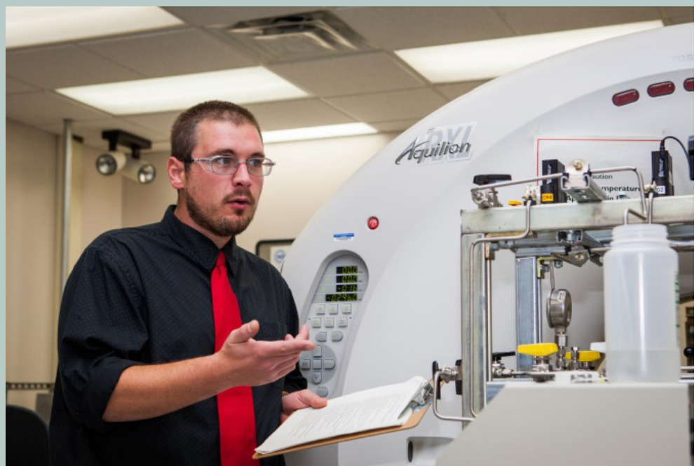
Dr. Dustin Crandall with an adapted medical computed tomography scanner used to study geologic core samples.
